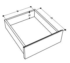
W x D x H A 310 x 385 x 80 mm W x D x H A 12.20 x 15.15 x 3.14 in.
