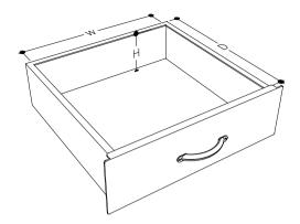
$\frac{W \times D \times H}{A 314 \times 390 \times 150 \text{ mm}}$  $\frac{W \times D \times H}{A 12.4 \times 15.3 \times 6 \text{ in}}$
